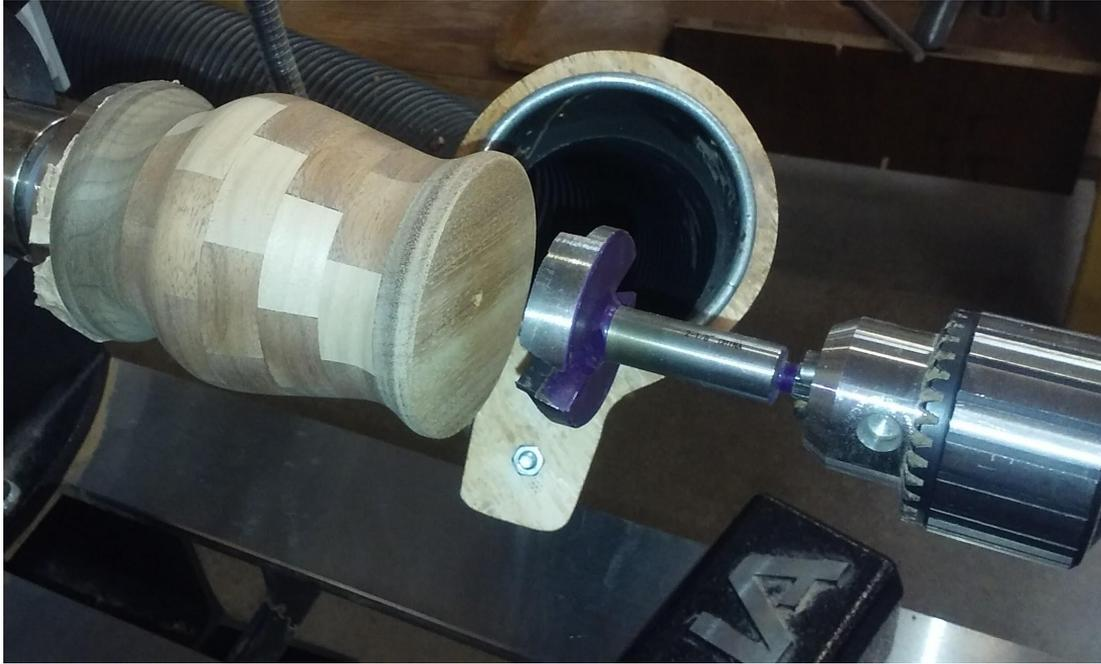
Once the shape is acceptable AND the outside is sanded, drill out the center. Use a 2 1/8" forstner bit
