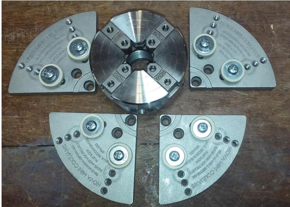
Cole jaws are used to mount the pencil holder with the top next to the head stock. The rubber pads will vary in color.
