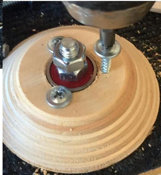
At this point, your bearing assembly is installed in the sanding disk, and this step is finished.
