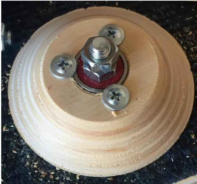
The next step will be to put a dense foam pad on the face of the rotary sanding disk.
