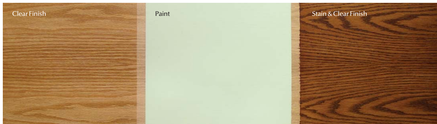
Finish on oak. On this oak panel, a clear finish was applied to the left section, paint to the middle section and a stain and clear finish to the right section.
