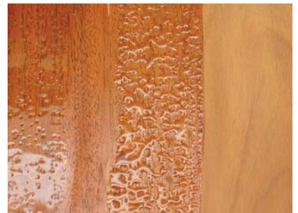
Fish eye. It's usually easy to spot the potential for fish eye by brushing the surface with mineral spirits, water or any stain. To avoid fish eye when the finish is applied, the silicone that causes the problem has to be washed out of the wood or blocked with shellac, or silicone has to be added to the finish to lower its surface tension.
