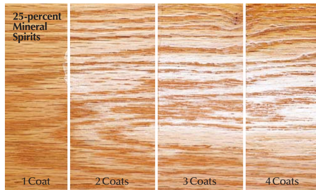
Thick mix. A thick mix of polyurethane and mineral spirits builds much more rapidly and is still thin enough for easy application.
